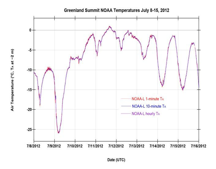
The plot shows temperature variations at Summit Station, Greenland (>3200 m or about 10,500 ft in elevation) during the major July 2012 ice sheet melt event observed by multiple satellites. Data from the NOAA Logan sensor at 2 m above the snow surface are shown with one and ten minute and one hour average air temperatures and document the approximately 6.5 hour long melt event on July 11th as well as the surprising warmth on adjacent days at that elevation.
