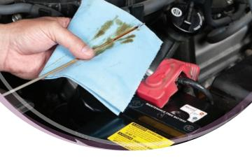
**Battery** The battery supplies power to the starter motor, acts as a voltage stabilizer and makes up for any shortfall when the alternator can't meet the vehicle's electrical needs. Inspect battery cable connections at every oil change and clean as needed. When inspecting a battery, always wear eye protection and gloves.
